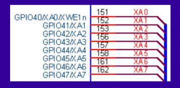
The keyboard connects to the Delfino EVB by External Bus using GPIO40-GPIO47.
