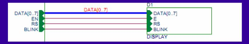
RS (function select) RS=0 command mode, RS=1 data mode – **GPIO57**
